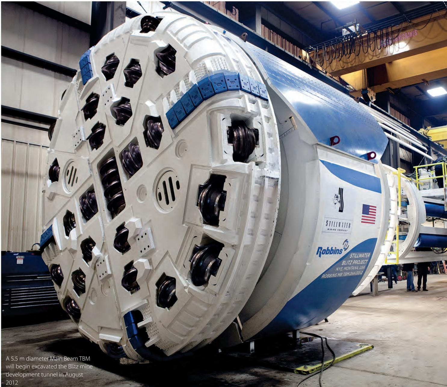
A 5.5 m diameter Main Beam TBM will begin excavated the Blitz mine development tunnel in August 2012
