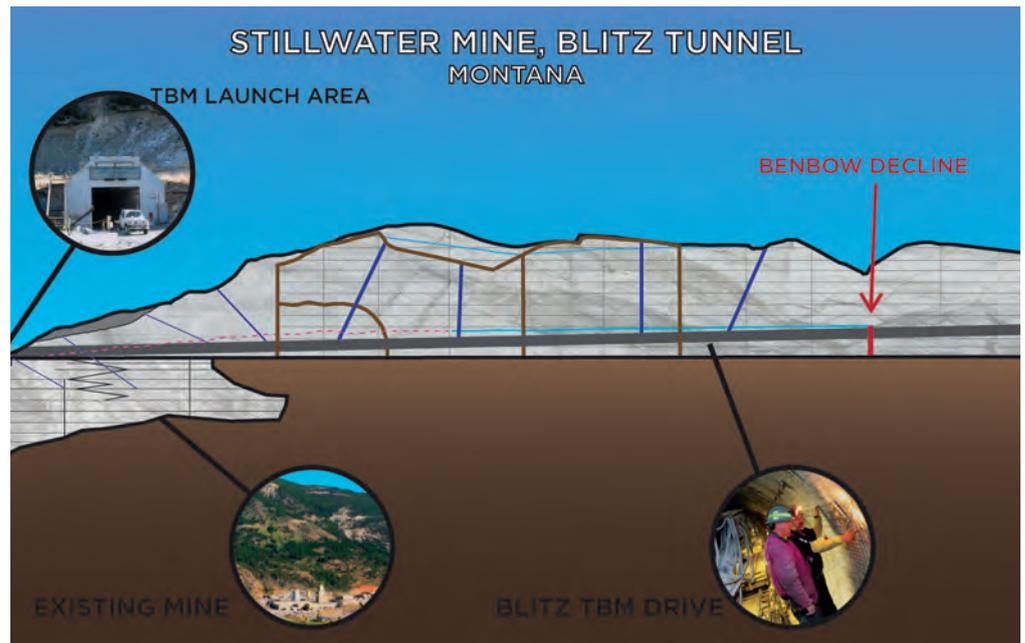
The Blitz tunnel drive will be at least 7.1 km in length and will cross several fault lines in mafic norite rock
