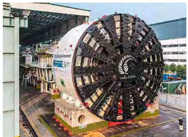
2 The cutting wheel of the EPB Shield for the twin-tube tunnels of the Waterview Connection Project has a diameter of 14.46 m and was tailored to the specific project conditions
