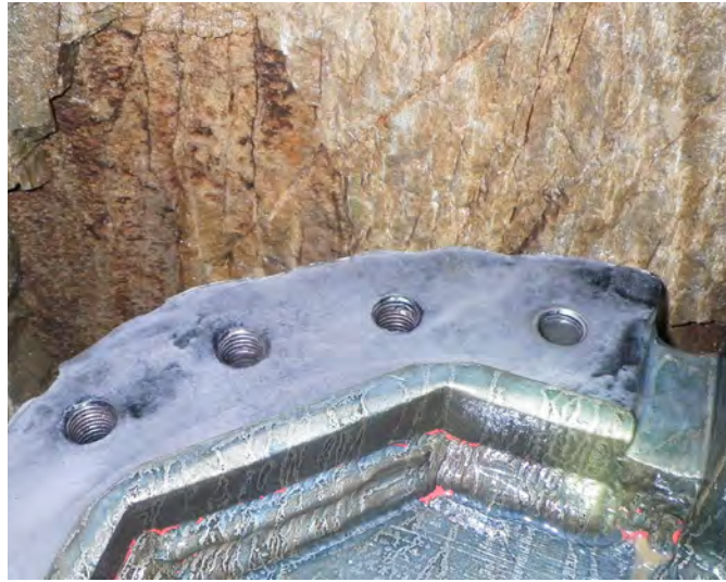
5 Räumer am Schneirad Scraper at the cutting wheel
