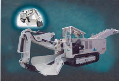
Loading capacity up to 2.5 m<sup>3</sup>/min
