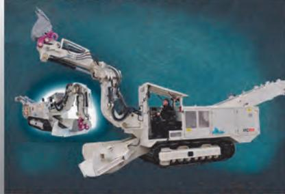
Loading capacity up to 2.5 m<sup>3</sup>/min
