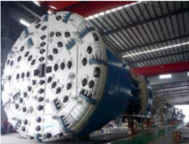
3 The Main Beams for China's West Qinling Tunnels were the first recent Robbins machines to be supplied with novel ring beam and materials handling systems, as well as mesh installation
