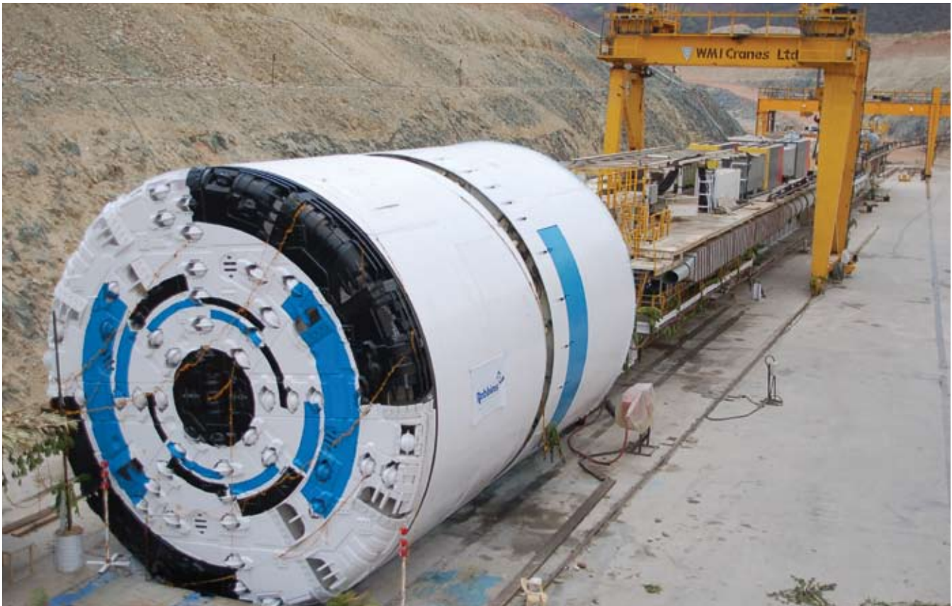
The TBM came equipped with 20-inch back-loading disc cutters for hard rock conditions, and a 360 degree probe drill
