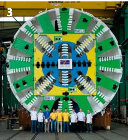
Double-track EPB TBM recently used for the São Paulo Metro Line 4
