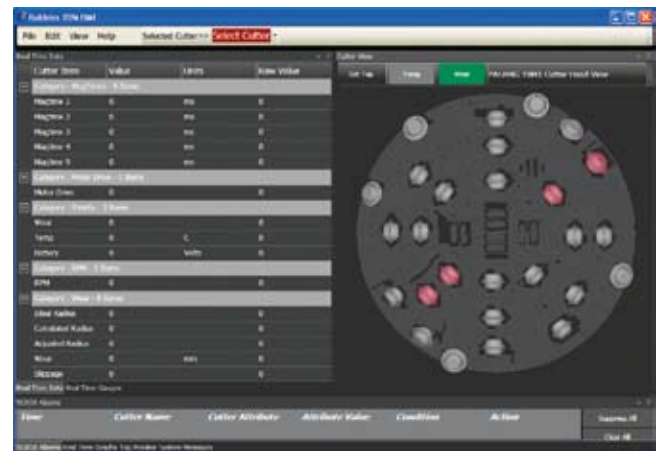
In this hypothetical illustration, an operator sees flagged cutters that are above a threshold limit indicating the presence of a fault zone
