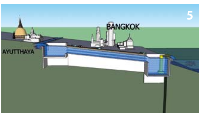
Major Flood Situation (both upper and lower decks using as flood drain tunnel)
