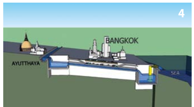
Moderate Flood Situation (upper deck using as motorway, lower deck draining out water)
