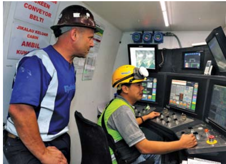
Wireless operator's cabs and touch screens in each TBM enable user-friendly tracking of all the machine's functions
