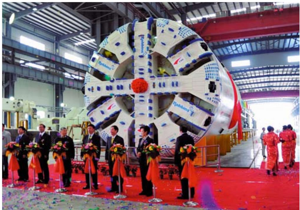
At China's Chengdu Metro, a 6.3 m diameter EPB was designed for glacial boulder, clay and sand
