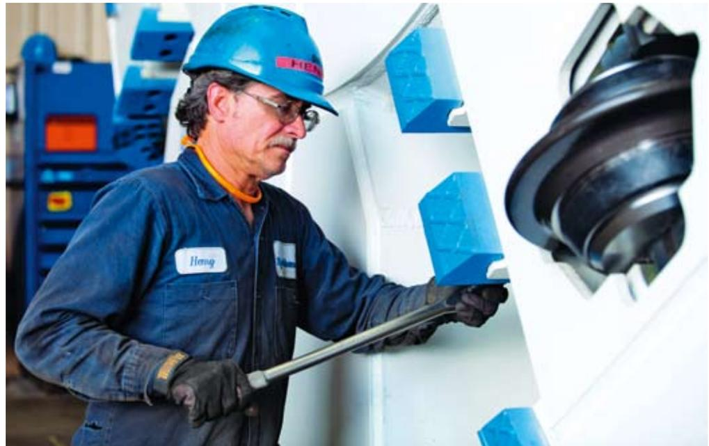
Mixed ground EPB cutterheads are often fitted with interchangeable knife bits and disc cutters
