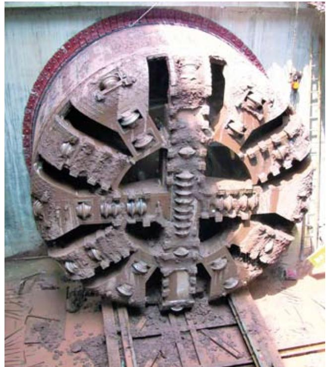
At China's Guangzhou metro, a mixed ground EPB excavated 4.5 km, with little to no visible cutterhead wear
