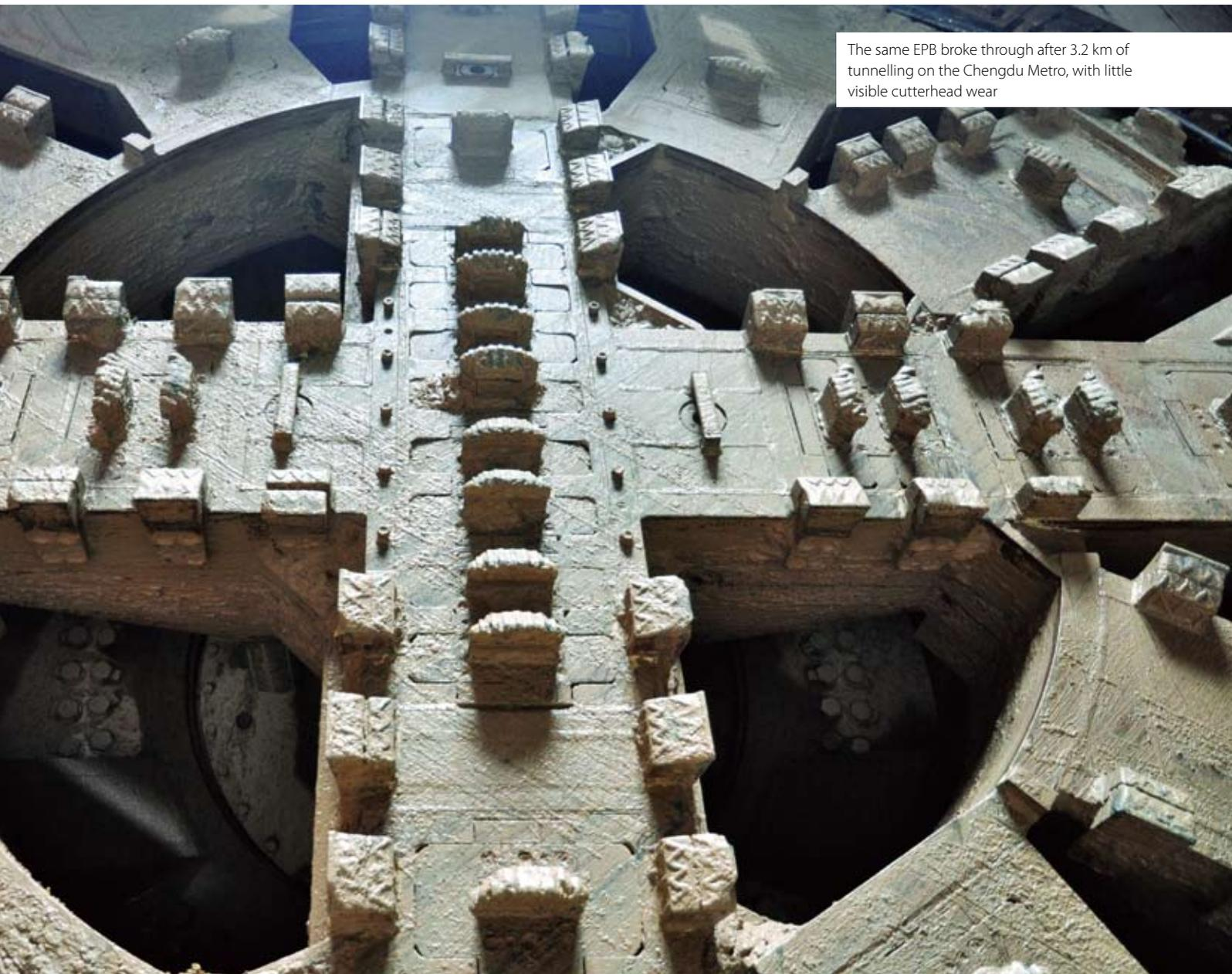
The same EPB broke through after 3.2 km of tunnelling on the Chengdu Metro, with little visible cutterhead wear
