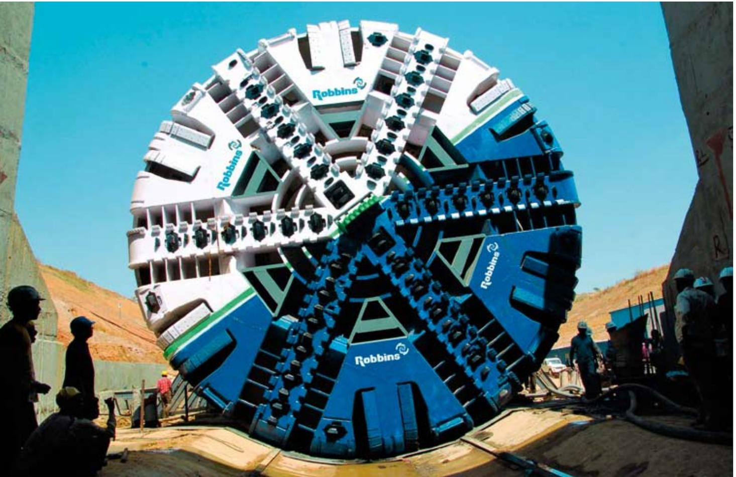
Protective wear plating, detection devices, and additives can minimize EPB cutterhead wear in even the most extreme conditions
